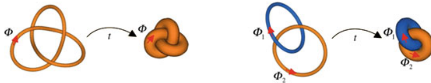
Fig. 1.20 Idealized magnetic relaxation of a trefoil knot and a Hopf link (image adapted from [44])
