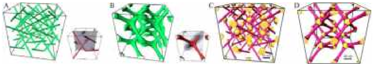
Fig. 72. Arrays of disclination lines in A blue phase I (BP I) and B blue phase II (BP II). Disclinations are visualized as iso-surfaces of degree of order S = 0.3 in BP I and S = 0.17 in BP II. Boxes constituted of 2 \times 2 \times 2 unit cells are shown (one unit cell length is 360 nm in BP I and 680 nm in BP II). Insets show the corresponding conventional unit cells. In the insets the projection of the director on the given plane is shown. Note the hyperbolic director pattern around the defects characteristic of -1/2 disclination lines. Circular director fields characterize arrays of double twist cylinders. C,D Three-dimensional BP colloidal crystals (particles in yellow). C Energetically favourable FCC colloidal crystal, 4 particles per unit cell in BP I, D the most energetically favourable BCC colloidal crystal with 2 particles per unit cell in BP II. In BP I, disclination lines are drawn as isosurfaces of degree of order S = 0.23 ( S_{\text{bulk}} = 0.40 ), particle radius is r = 70 nm. In BP II, disclination lines are visualized as isosurfaces of S = 0.1 ( S_{\text{bulk}} = 0.26 ), r = 50 nm. In all cases 2 \times 2 \times 2 unit cells have been shown better to illustrate the structure. Source: C,D reproduced from [682].
