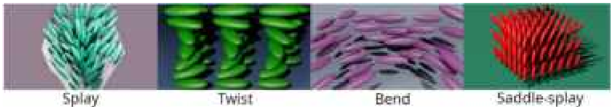
Fig. 31. Splay, twist, bend and saddle-splay distortions of a nematic liquid crystal.
