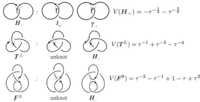
**Figure 3.** The Jones polynomial of the (negative) Hopf link  $V(H_-)$ , left-handed trefoil knot  $V(T^L)$ , and figure-of-eight knot  $V(F^8)$ .
