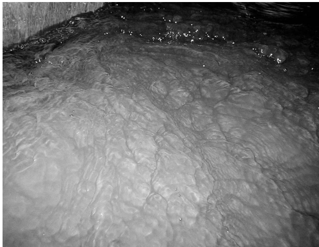
Fig. 1: The free surface of a turbulent flow. On the surface a network of grooves or “scars” is visible.
